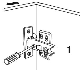
2. The horizontal adjustment screw adjusts the door forward or backward.
